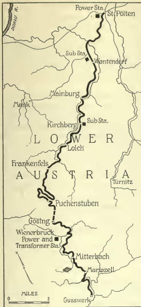
FIG. 482. ELECTRIFIED LINES OF THE ST. PÖLTEN-MARIAZELL-GUSSWERK RAILWAY
